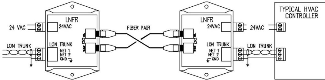
The LNFR single channel fiber repeater is used in a point to point application to extend the physical twisted pair network up to 2.5 km. The LNFR acts as a repeater only, and is completely transparent to the network. Any communication received on the near side of the free topology network will be propagated to the far side via fiber optic cable, where the twisted pair signal will be regenerated on the far side of the network.
